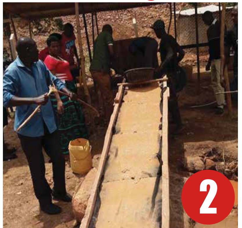
Pour crushed ore in the sluice box and wash in water
