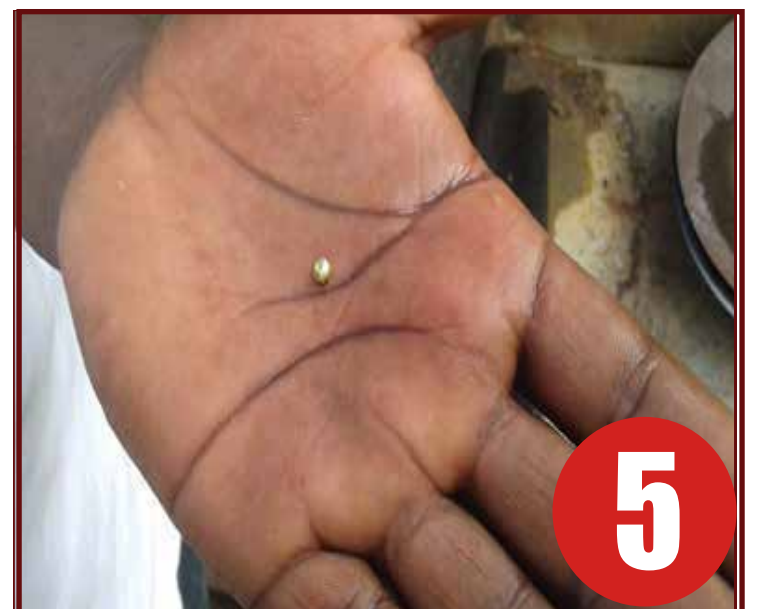
The liquid is then cooled to form a solid mass of gold
