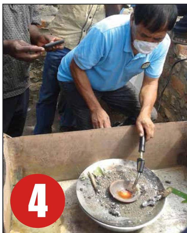
Add borax to the concentrate and heat. This is direct smelting
