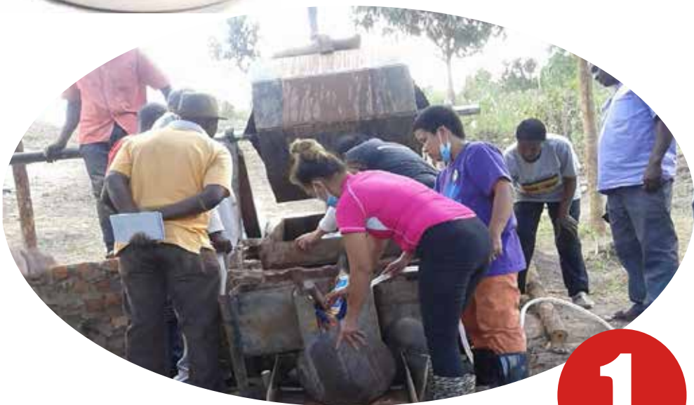
Crush the ore to liberate gold particles through wet milling
