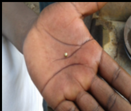
[LEFT] Borax added to the gold concentrate on spoon and heated [RIGHT] A piece of pure gold after heating with borax
