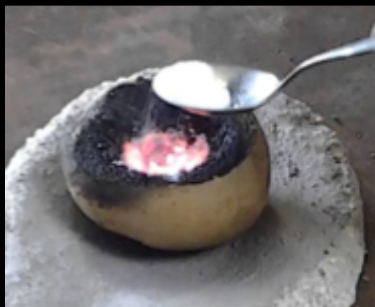
[LEFT] Borax added to the gold concentrate on spoon and heated [RIGHT] A piece of pure gold after heating with borax
