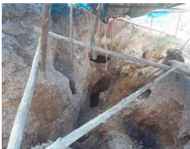
Poor mining practices: Mining tunnels constructed by Gold miners in Mubende are a risk to the miners and pose a long term environmental threat.
