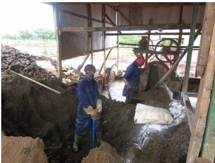
Carbon on Pulp (CoP) Process: Workers introducing lime into the earth material containing the gold ore before introducing cyanide
